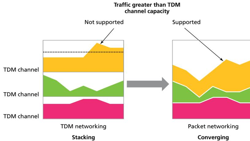
New Packet Optical Transport Systems and microwave packet radios offer resiliency, increased bandwidth capacity, effectiveness and flexibility to allow true network convergence. WDM is added in areas where fiber capacity is exhausted to cost-effectively increase bandwidth capacity. The addition of Zero Touch Photonics capabilities further simplifies WAN operations.
