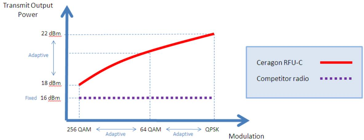
**Figure 2: Adaptive-Modulation with Adaptive-Power feature Versus Adaptive-Modulation with a Fix Power level, over 18-23 GHz link**
