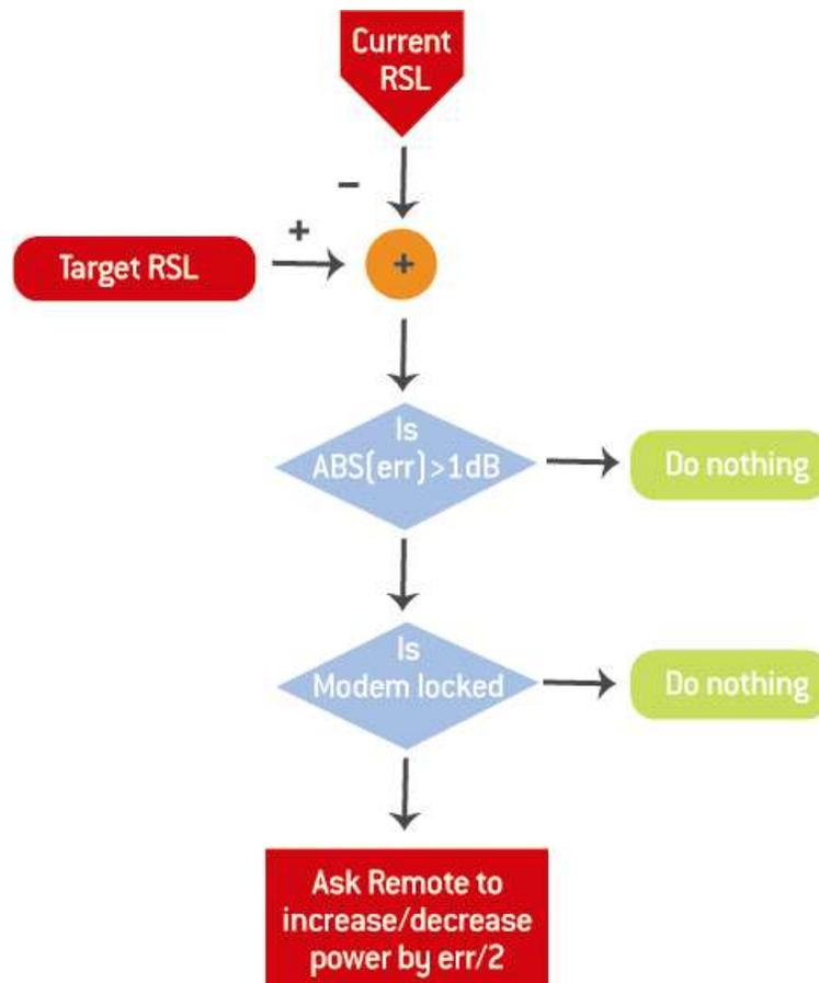
Figure 3: Diagram chart explaining the behavior of ATPC algorithm
