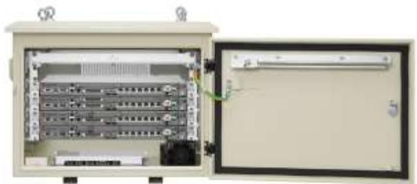
Outdoor enclosures, which house the equipment and alleviate the need for expensive and scarce indoor space, have become a viable and cost-saving alternative. This paper discusses the problems and costs of the traditional in-building solution, introduces the Ceragon FibeAir Outdoor Enclosure, and surveys the advantages and challenges of the outdoor enclosure approach.
