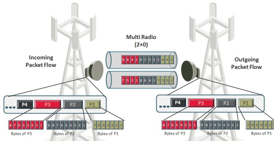
Figure 3: Multi-Carrier ABC traffic distribution across multiple wireless links
