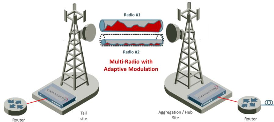
**Figure 4: Multi-Carrier ABC’s independent carriers using adaptive modulation**
