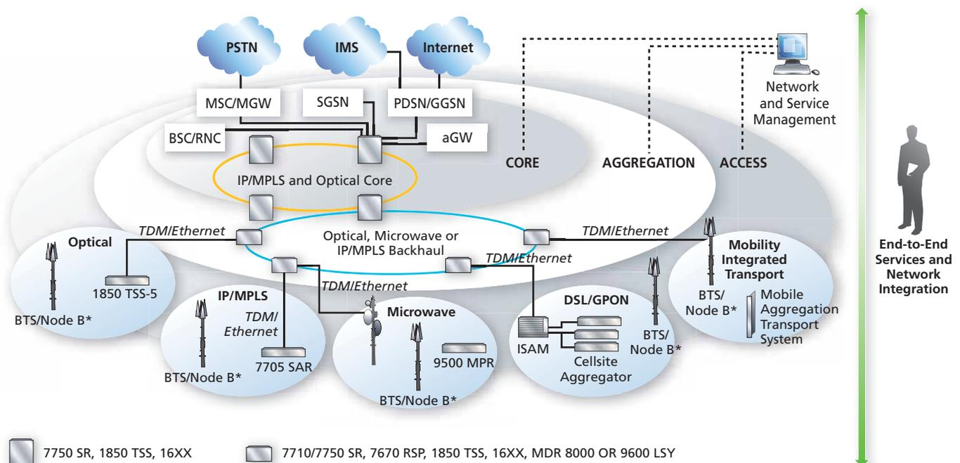
\* SUPPORT OF MULTI-GENERATIONAL WIRELESS NETWORKS USING ANY BTS/NODE B (CDMA BTS, GSM/GPRS BTS, UMTS, WIMAX, EVDO/HSPA, BSR FEMTO, LTE)
