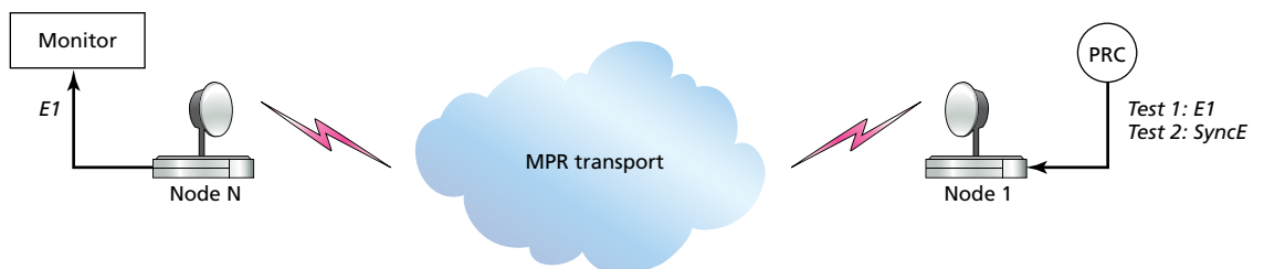
Figure 6. Test set 1: synchronization measurement for an egress E1 data line, N = 20
