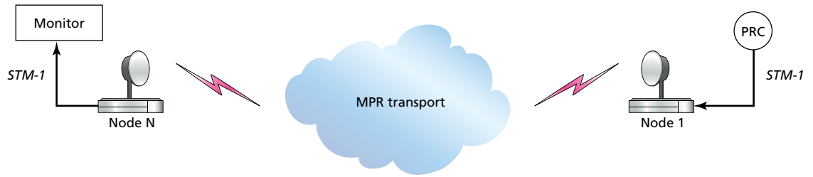
Figure 7. Test set 2: synchronization measurement for STM-1, N = 20
